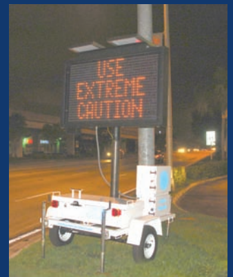
This is a variable message sign used to advise the public of traffic concerns and alert the motorist to watch for pedestrians.
